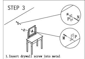
bracket and into drywall anchor.
