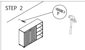
1. Use a light hammer to tap anchor into hole.
