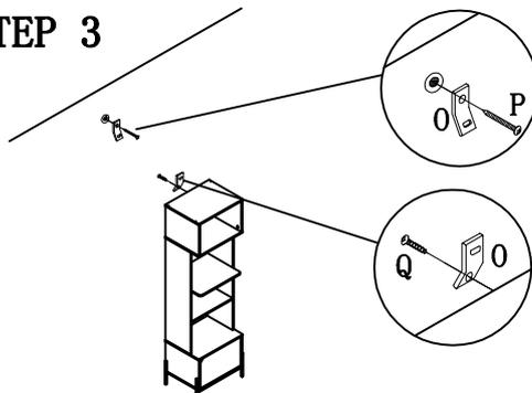
1. Insert drywall screw into metal bracket and into drywall anchor.
