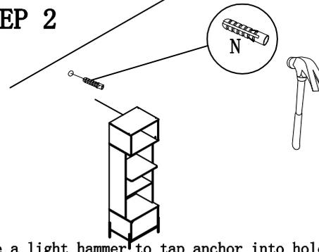
1. Use a light hammer to tap anchor into hole.
