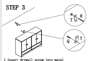
bracket and into drywall anchor.
