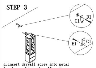
bracket and into drywall anchor.
