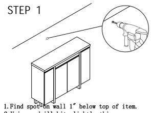
1. Find spot on wall 1" below top of item 2. Using a drill bit slightly thinner than anchor, drill hole into drywall.
